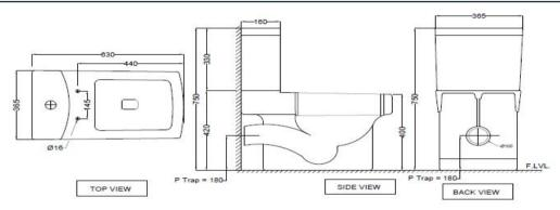
ALL DIMENSIONS ARE IN MM. (TOLERANCE ± 5 MM)
