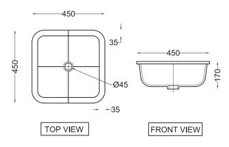
ALL DIMENSIONS ARE IN MM. (TOLERANCE ± 5 MM)
